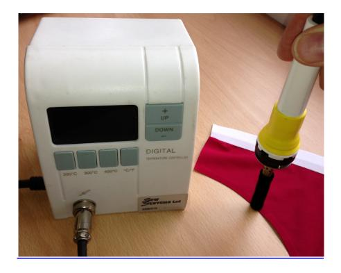
The SSM310 Spot tacking gun is for tacking seams over in selected areas that have the adhesive already applied, before running through the bonding machine.
