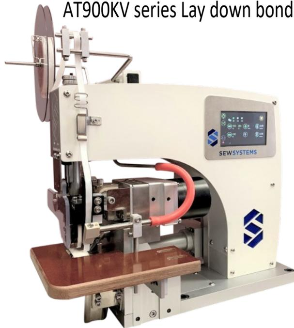
This machine applies heat with Heated Belts, hot air and can be converted to use all the below methods of application. independently driven heated belts, Drop roller foot belts, silicon rollers in any combination
