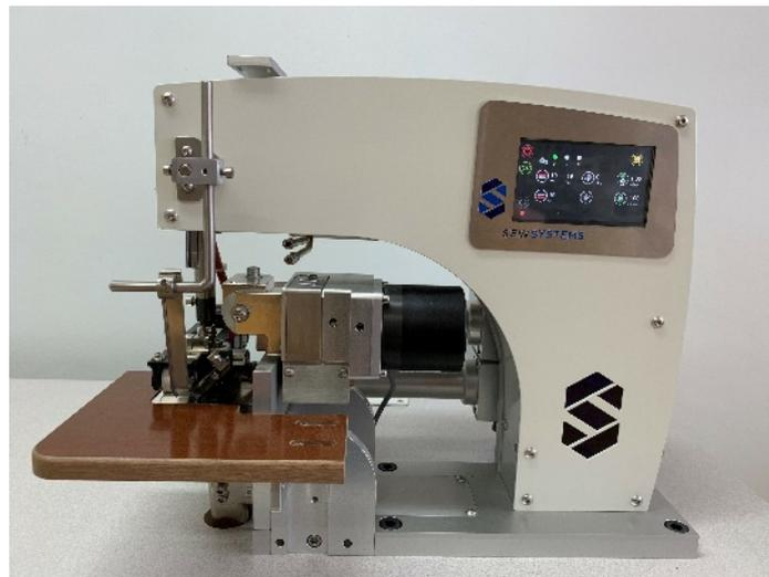
This machine applies heat with Heated Belts, hot air and can be converted to use all the below methods of application. independently driven heated belts, Drop roller foot belts, silicon rollers in any combination
