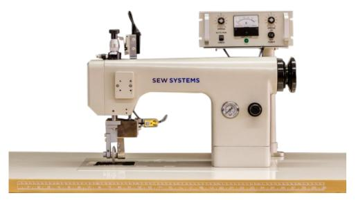
Ultrasonic machine for edge finishing/cutting/sealing/ embossing textiles, without puncturing. This machine is used to ultrasonically cut and join two pieces of at least 60% manmade fabrics together. Ideal for non wovens and PPE, face masks etc
