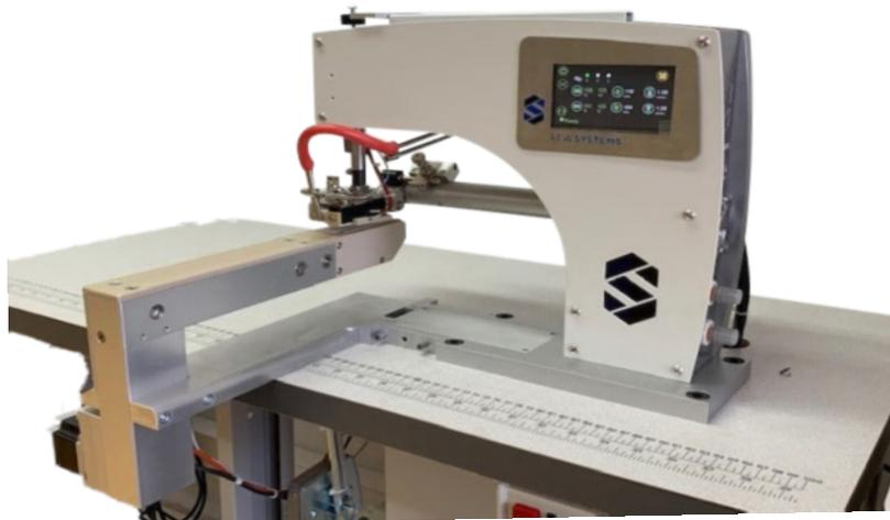
This machine applies heat with Heated Belts, hot air and can be converted to use all the below methods of application. independently driven heated belts, Drop roller foot belts, silicon rollers in any combination
